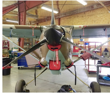
Siai Marchetti 1019 Engine Plugs, Prop Tie-Exhaust Covers
