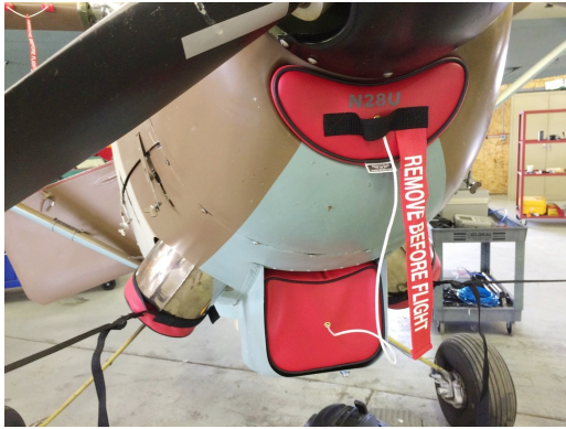
Siai Marchetti 1019 Engine Plugs, Prop Tie-Exhaust Covers
