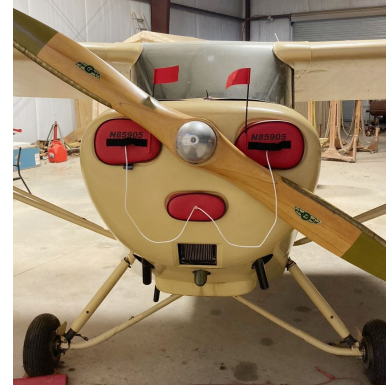
Aeronca 11AC Engine Inlet Plugs
