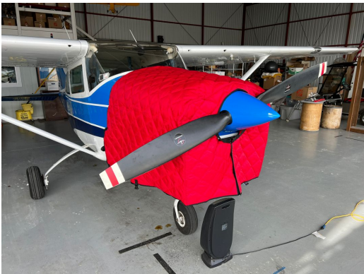
Insulated Hangar Blanket on Cessna 182
