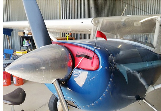
Cessna 150J Engine Inlet Plugs
