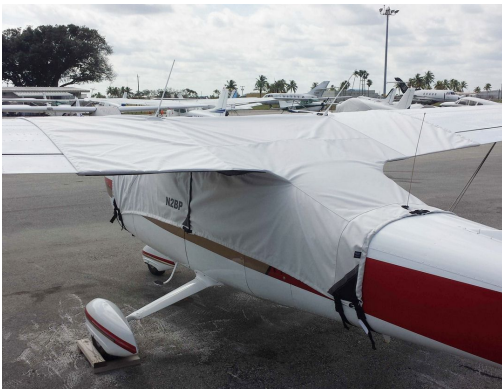
Cessna 177B Cardinal Canopy Cover, Over-Top, Ext. to cover gas caps, 6" fwd extension.
