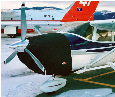
Cessna 182 Skylane Insulated Engine Cover, Fully Enclosed
