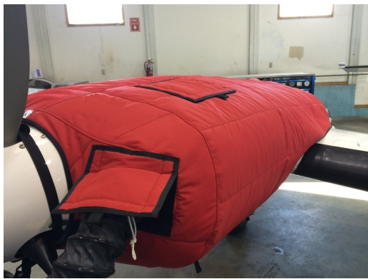
Cessna 402 Insulated Engine Cover with Heater
