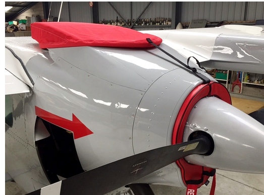
Cessna 337 Skymaster Aft Engine Inlet Cover, hoop type, & outlet plugs (SOLD SEPARATELY)
