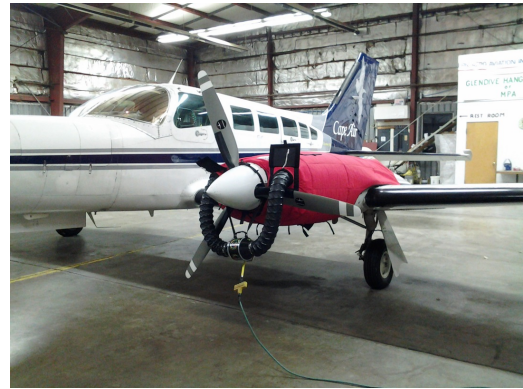
Cessna 402 Insulated Engine Cover with Heater
