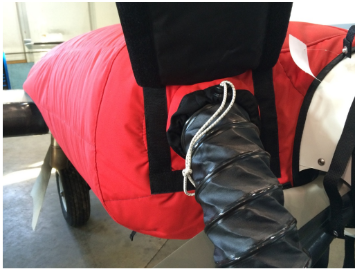
Cessna 402 Insulated Engine Cover with Heater
