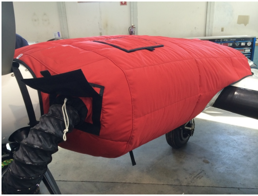
Cessna 402 Insulated Engine Cover with Heater
