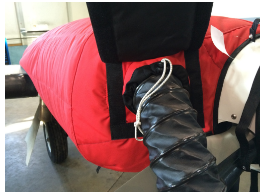
Cessna 402 Insulated Engine Cover with Heater
