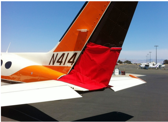
Cessna 414 Rudder Openings Cover (bird barrier)
