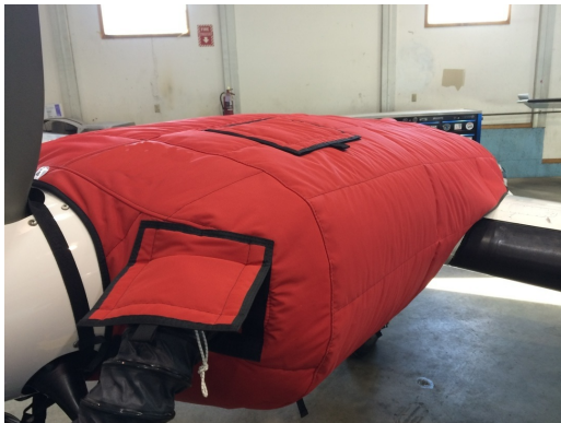
Cessna 402 Insulated Engine Cover with Heater
