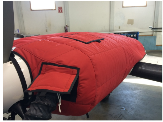
Cessna 402 Insulated Engine Cover with Heater
