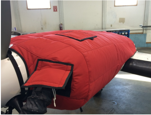
Cessna 402 Insulated Engine Cover with Heater
