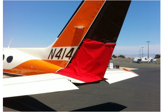
Cessna 414 Rudder Openings Cover (bird barrier)
