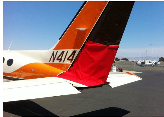
Cessna 414 Rudder Openings Cover (bird barrier)
