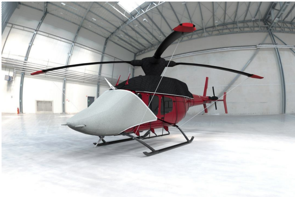
Bell 429 Cockpit/Nose Cover, Engine Cover, etc.
