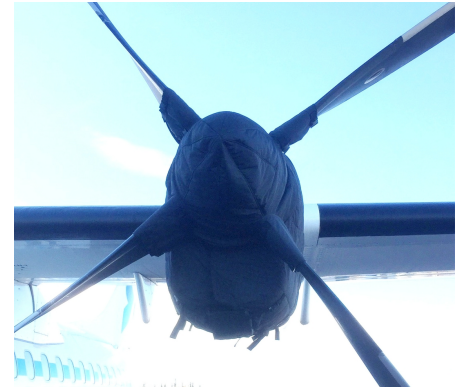
ATR-72-202 Insulated Engine & Prop Hub Covers
