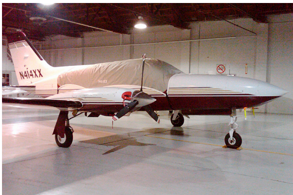
Cessna 414 Canopy Cover and Engine Inlet Plugs
