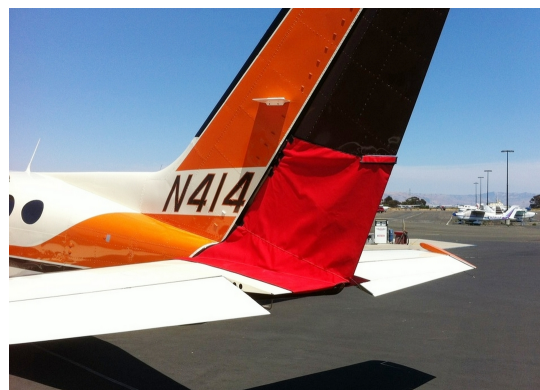
Cessna 414 Rudder Openings Cover (bird barrier)
