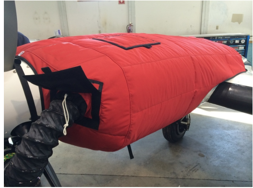
Cessna 402 Insulated Engine Cover with Heater
