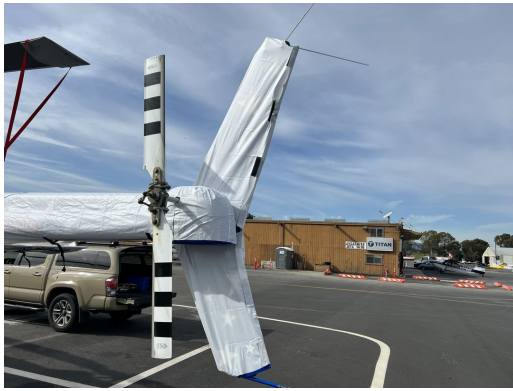
Bell 505 Tailboom & Stabilizer Covers, test fit cover
