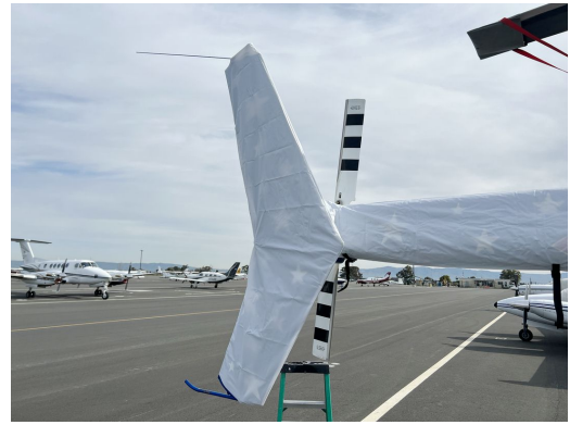
Bell 505 Tailboom & Stabilizer Covers, test fit cover
