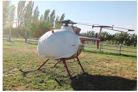
MD500D Bubble Cover with Intake Add-On
