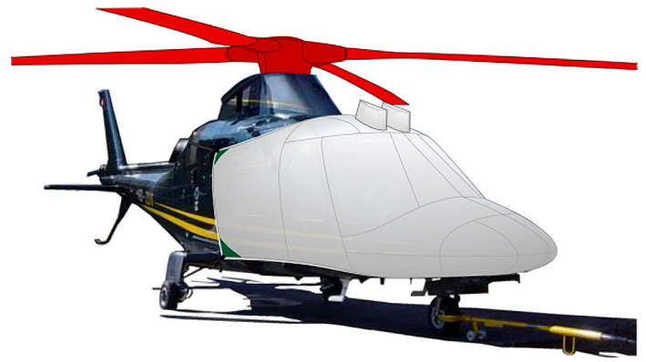
Agusta 109 Bubble, Rotor Hub & Blade Covers (illustration)
