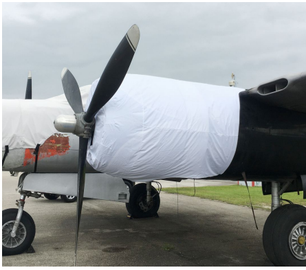
Douglas A-26 Engine Cover, test fit cover
