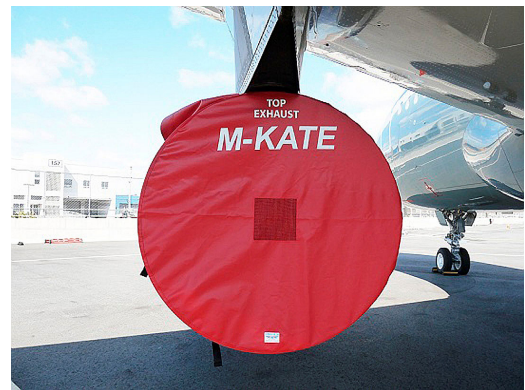
Airbus A319 Intake/Exhaust Covers set, IAE V2500
