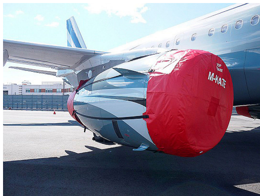
Airbus A319 Intake/Exhaust Covers set, IAE V2500
