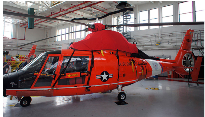
MH-65C Rotor Hub, Swash Plate Aperture, Engine Area Cover set, P/N: A365-210
