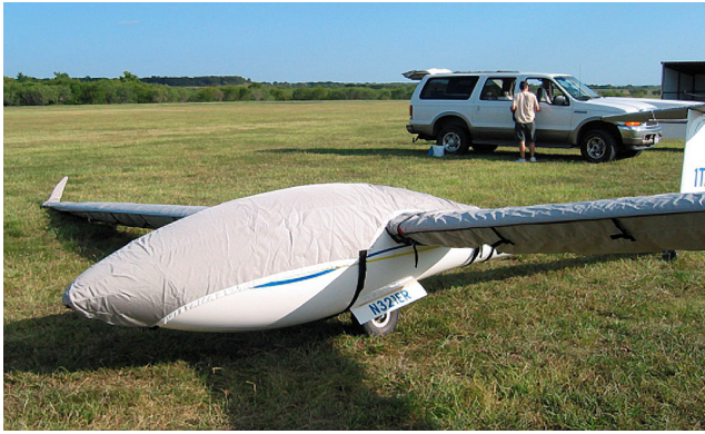
Canopy/Nose Cover, Wings and Horizontal Stab Covers
