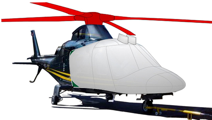
Agusta 109 Bubble, Rotor Hub & Blade Covers (illustration)
