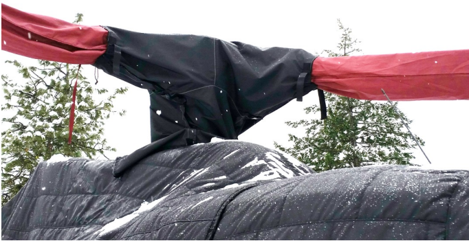
Main Rotor Hub Cover with swash plate extension.
