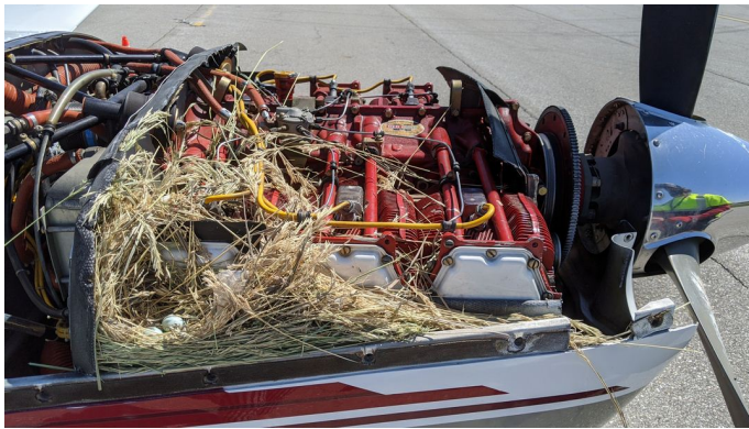
ENGINE PLUGS PREVENT BIRD NEST FOD. Piper Saratoga Engine Cowling Bird's Nest Piper Apache Engine Plugs, Prop Covers
