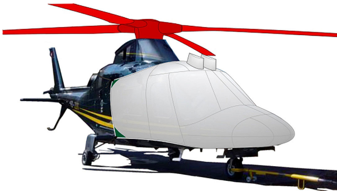
Agusta 109 Bubble, Rotor Hub & Blade Covers (illustration)
