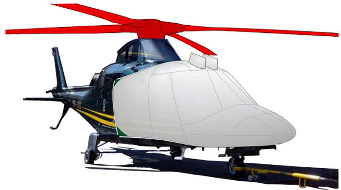
Agusta 109 Bubble, Rotor Hub & Blade Covers (illustration)
