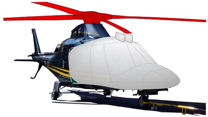
Agusta 109 Bubble, Rotor Hub & Blade Covers (illustration)
