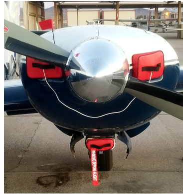
Piper Aztec Engine Inlet Plugs with lower cowling induction air inlet plug.
