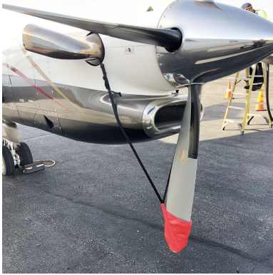
Beech King Air 350 Prop Tie-Downs
