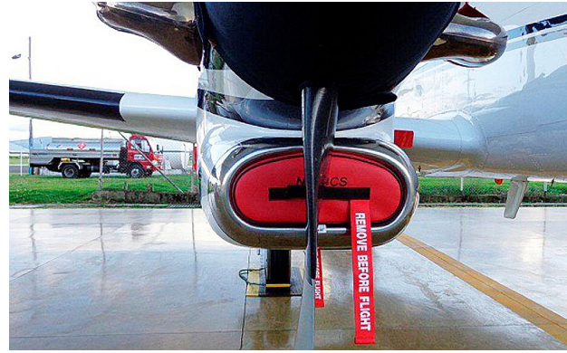
Beech King Air C90B Main Engine Inlet Plug
