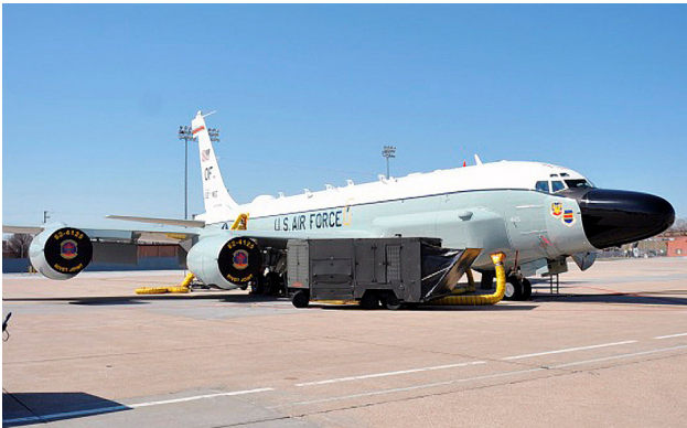
KC-135 “Tambourine” style, Double Fold Intake Covers at Offutt AFB
