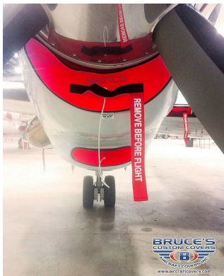
Engine and Oil Cooler Inlet Plugs ENGINE PLUGS PREVENT BIRD NEST FOD. Piper Saratoga Engine Cowling Bird's Nest
