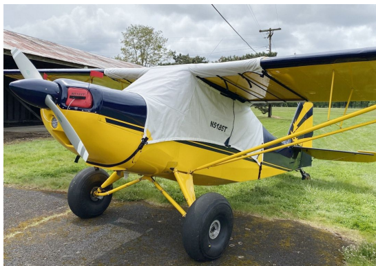
American Champion Citabria canopy cover over the top style, extends to cover gas caps, Engine Plugs
