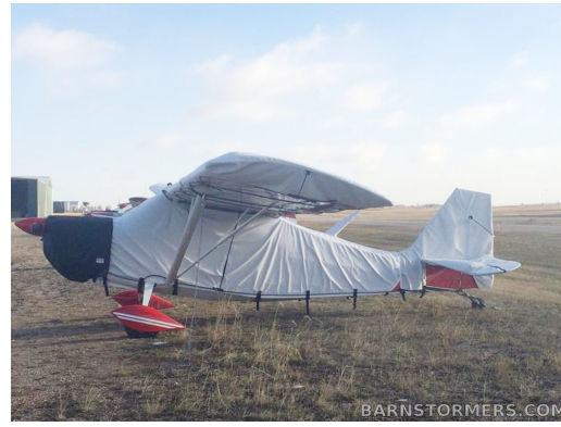
Bellanca Citabria Extended Canopy Cover (extended to tail), Empennage, Wing, Insulated Engine Cover
