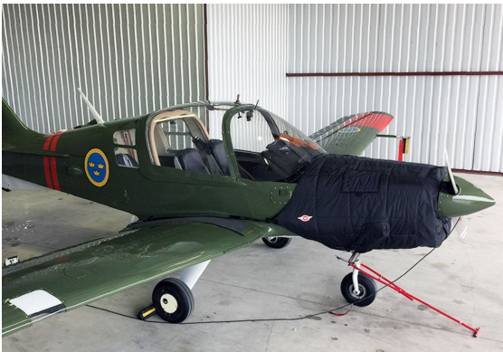
Scottish Aviation Bulldog Insulated Engine Cover
