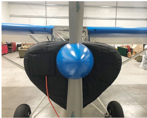
Bearhawk Patrol Insulated Engine Cover, with electric heater access flap Bearhawk Engine Cover (test fit), Insulated Prop Cover
