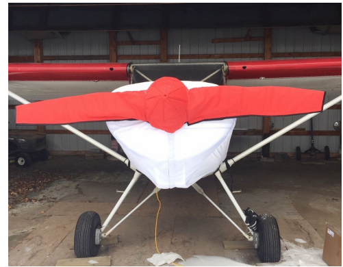
Bearhawk Patrol Insulated Engine Cover, with electric heater access flap Bearhawk Engine Cover (test fit), Insulated Prop Cover
