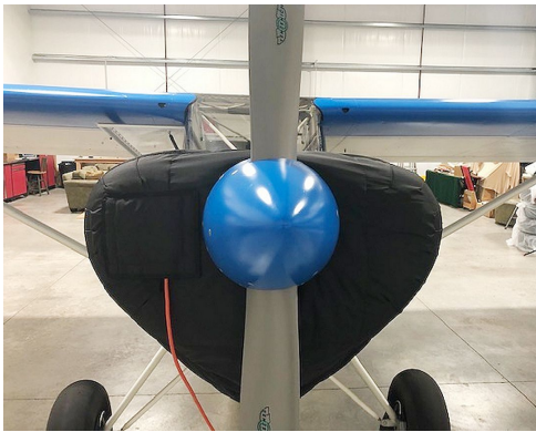
Bearhawk Patrol Insulated Engine Cover, with electric heater access flap
