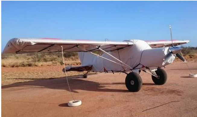
Maule M7-235 Extended Canopy, Wing, Engine & Empennage Covers
