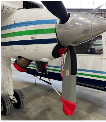
Britten-Norman Islander Engine Inlet Plugs & Prop Tie
