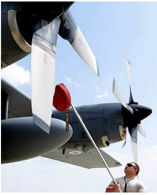
C-130 Inlet Plugs (and the clever gentleman installing the plug)
