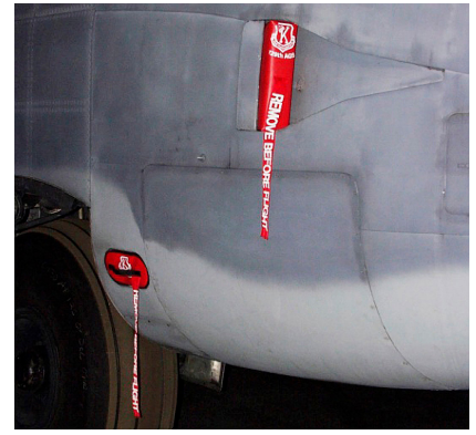
C-130 Heat Exchanger & Exhaust Plugs
