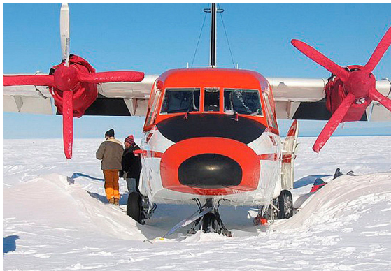
Casa 212 Insulated Engine & Propellor/Spinner Covers
