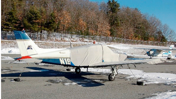
Beech Sierra Prop, Engine, Extended Canopy, Wing, Tailcone, and Horizontal Stab Covers.
