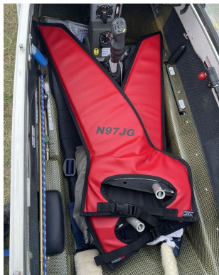
Schempp-Hirth Ventus-2B winglet/wingtip pads
