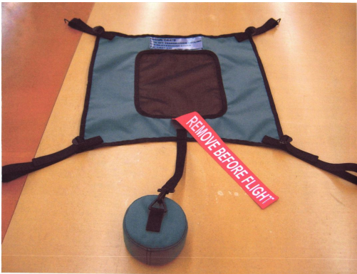
Boeing Vertol CH-47 Chinook Aft Transmission Cooling Fan Inlet/Exhaust Cover
