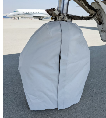
CJ1 Nose Gear Tire Cover, test fit
