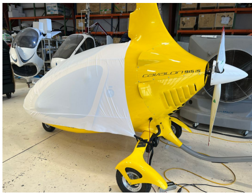
Autogyro Cavalon Canopy/Nose Cover, test fit cover
