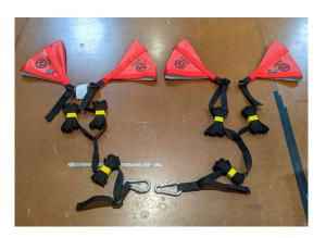
Dornier 328 Turboprop, C-146A Wolfhound Prop-Tie Downs, Turbo Prop Engines
