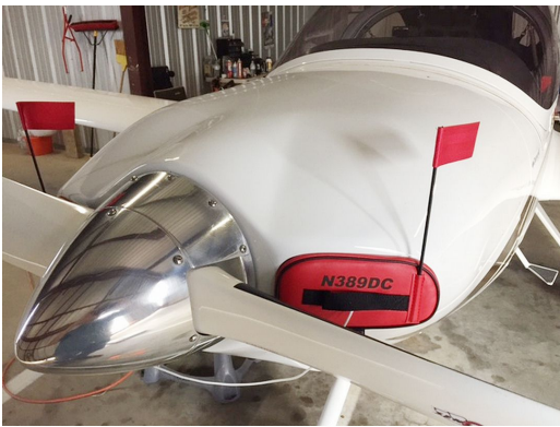
Diamond DA-20-C1 Engine Inlet Plugs ENGINE PLUGS PREVENT BIRD NEST FOD. Piper Saratoga Engine Cowling Bird's Nest
