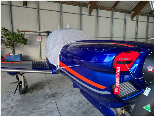
Diamond DA-50 Canopy Cover, Engine Plugs
