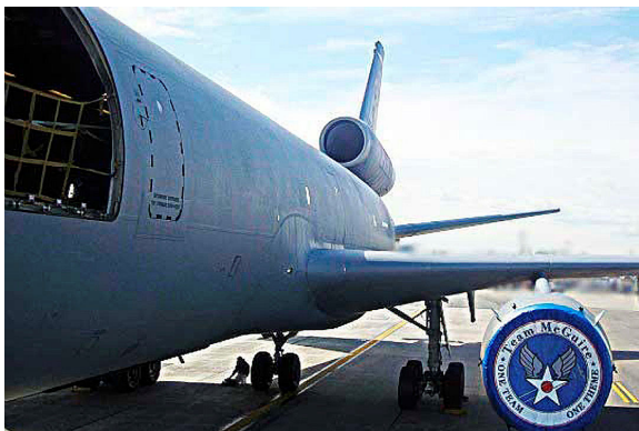
KC-10 Intake Cover at McGuire AFB, NJ
