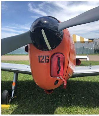
De Havilland Chipmunk Engine Plug ENGINE PLUGS PREVENT BIRD NEST FOD. Piper Saratoga Engine Cowling Bird's Nest
